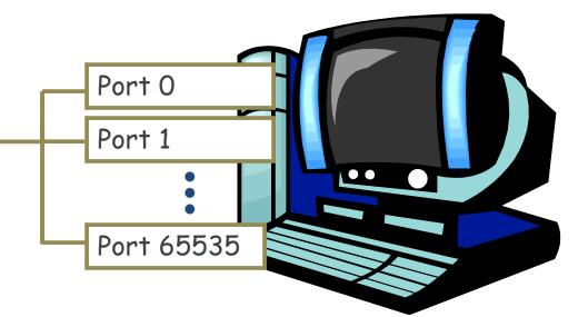
A socket provides an interface to send data to/from the network through a port
